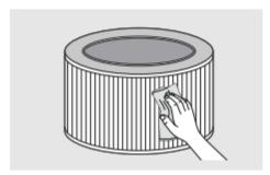
Gently brush off the collected dust on the surface of the prefilter with dry cloth, or vacuum cleaner for optimal performance.
