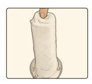
5. Tuck the excess filter fabric remaining over the valve between the wire clips of the frame.
