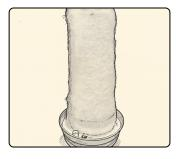
4. Slide the filter over the frame. Pull the filter over the sealing ring all the way to the valve body. Make sure the seal stays in the correct position.
