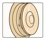
6. Put the valve back in place. Rotate the valve in the duct so that it sits tightly. Position the valve plate so that the draft-reducing air deflector is at the bottom.
