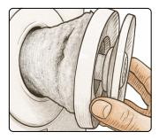
1. Take a firm grip on the valve body located under the valve plate and carefully pull the valve out. Remove the dirty filter.
