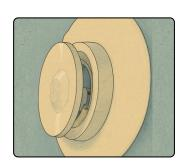
3. When the plate has been turned half a turn, the valve does not close completely as the temperature drops, but always remains open.
