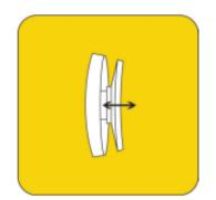
3. After turning the plate half a turn, the valve will not close as the temperature decreases but will remain slightly open by approximately 2mm.
