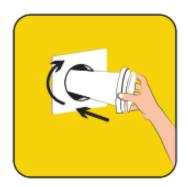
6. Place the valve back into position Rotate the valve within the passage pipe to ensure a proper seal.
