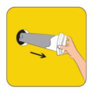
1. Take a grip from the valve body under the plate and carefully pull the valve out. Remove the dirty filter.
