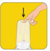
5. Push the excess filter fabric remaining above the valve into the gaps between the frame wires.
