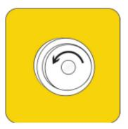
2. When the plate clicks, turn the plate at least half a turn counterclockwise to open it.
