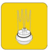
Ensure that the O-sealing ring is in the position indicated in the image.
