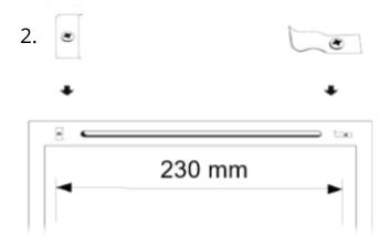
On the other side of the sash, the filter brackets are screwed in place on both sides of the slot, 230 mm apart from each other.
