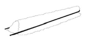
The filter is pulled over the support grid and pressed onto the mesh using a wire clip.
