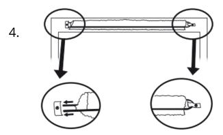
The open end of the arch is first pushed under the bridge-like holder and finally locked in place with the holder at the other end.
