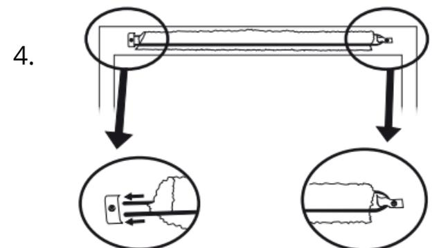
The open end of the arch is first pushed under the bridge-like holder and finally locked in place with the holder at the other end.
