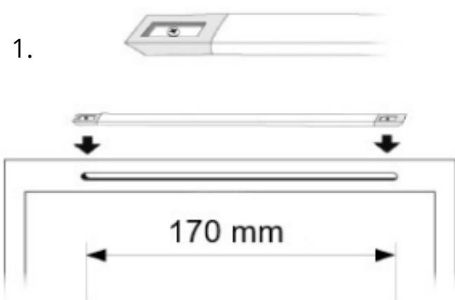
A slot approximately 8-10 mm x 170 mm in size is milled into the inner sash, preferably in the upper part of the sash, allowing the incoming air to be directed upwards. The infinitely adjustable vent is attached with screws over the slot so that the flap opens upwards.
