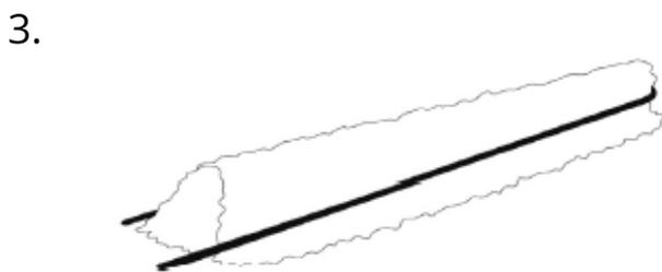
The filter is pulled over the support grid and pressed onto the mesh using a wire clip.
