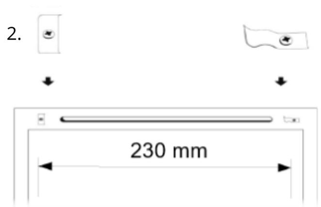
On the other side of the sash, the filter brackets are screwed in place on both sides of the slot, 230 mm apart from each other.
