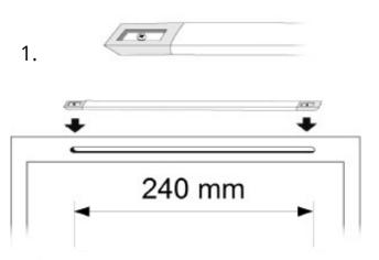
A slot approximately 8-10 mm x 240 mm in size is milled into the inner sash, preferably in the upper part of the sash, allowing the incoming air to be directed upwards. The infinitely adjustable vent is attached with screws over the slot so that the flap opens upwards.
