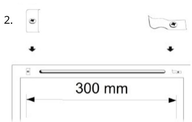
On the other side of the sash, the filter brackets are screwed in place on both sides of the slot, 300 mm apart from each other.
