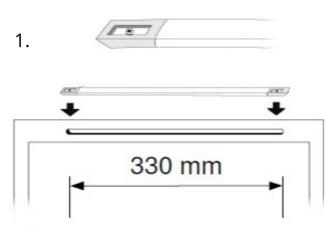
A slot approximately 8-10 mm x 330 mm in size is milled into the inner sash, preferably in the upper part of the sash, allowing the incoming air to be directed upwards. The infinitely adjustable vent is attached with screws over the slot so that the flap opens upwards.
