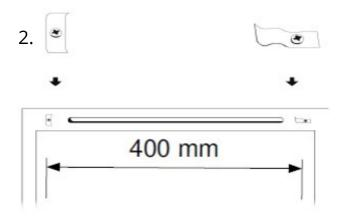
On the other side of the sash, the filter brackets are screwed in place on both sides of the slot, 400 mm apart from each other.
