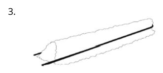
The filter is pulled over the support grid and pressed onto the mesh using a wire clip.
