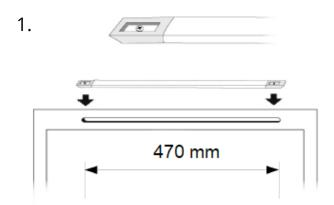
A slot approximately 8-10 mm x 470 mm in size is milled into the inner sash, preferably in the upper part of the sash, allowing the incoming air to be directed upwards. The infinitely adjustable vent is attached with screws over the slot so that the flap opens upwards.
