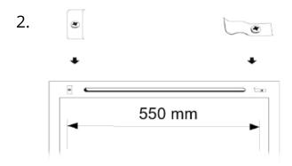
On the other side of the sash, the filter brackets are screwed in place on both sides of the slot, 550 mm apart from each other.
